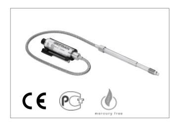
The KE Series are for use in high temperature applications where the process temperatures may reach 538°C (1000°F) such as high temperature engineered polymers. The K Series utilizes standard melt pressure principles and construction, but uses a near incompressible NAK (Sodium Potassium) for pressure transmission. The K Series strain sensing technology is bonded foil strain gage.
